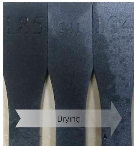
Figure 10 - Drying of brake fluid on tensiles
