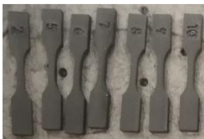
Figure 5 - Tensiles that were in contact with motor oil in Test 1- Type V
