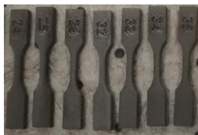
Figure 6 - Tensiles that were in contact with Valvoline Gear Oil in Test 1- Type V
